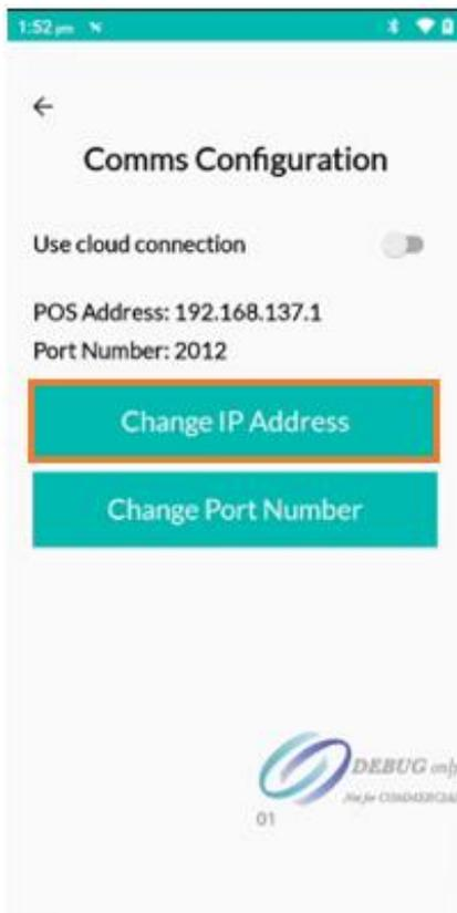
4. By default, the Linkly software listens for terminal communications on port 2012, leave this on 2012.
